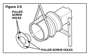
2. Remove the outer wheel bearing from the ring gear hub.
