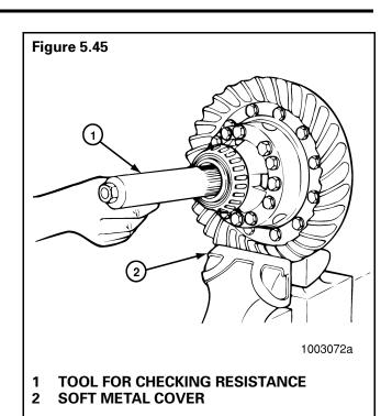
d. Attach a torque wrench to the nut of the tool and rotate the differential gears. As the differential gears rotate, read the value indicated on the torque wrench. **Figure 5.46**.
