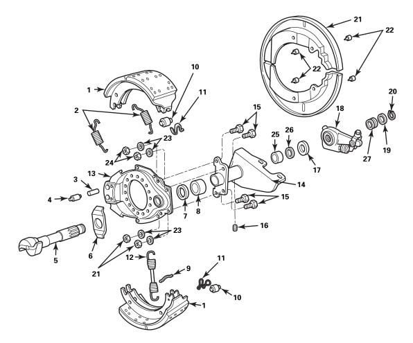
16.5-Inch Q Plus<sup>™</sup> Cam Brake with a Stamped Spider
