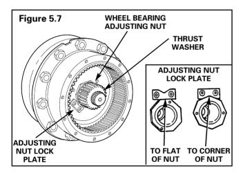
8. If necessary, tighten the adjusting nut to align the lockplate holes with the threaded holes in the ring gear hub. Do not loosen the adjusting nut.
