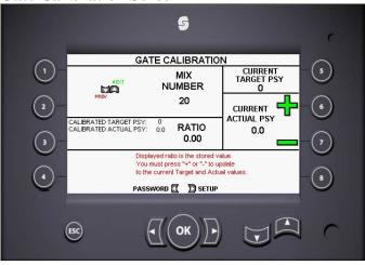
This screen is used for calibrating the Mix ratio.
