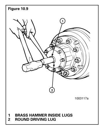
b. Hit the end of the drift with a large hammer (5 to 6 pounds, 2.3 to 2.7 kg) to loosen the axle shaft and tapered dowels from the hub. Figure 10.9. 8. Air Hammer Method:
