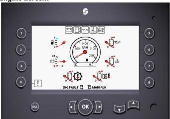
The Engine screen displays information from the engine ECM. If the ECM detects a problem the fault indicator will flash red, pressing button 4 will switch to the Engine Faults screen.
