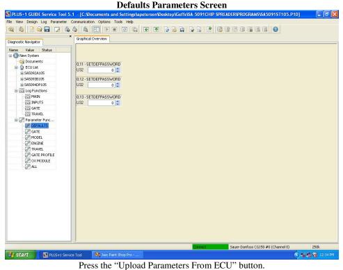
Enter 2012 into the SETDEFPASSWORD BOXES and press the "Download Parameters to ECU" button to reset parameters to the factory defaults.
