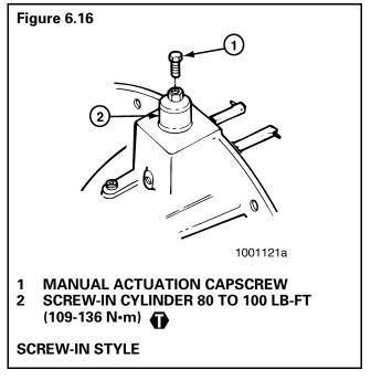
8. Snap the shift collar into the fork and engage the shift collar splines with the splines of the differential case. Use the manual actuation capscrew to move the shift collar splines into the differential case splines. Refer to "Manual Engaging Method."
