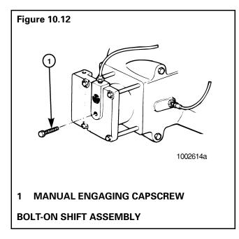
b. Turn the capscrew to the right until the head is approximately 0.25 to 0.50 inch (6.4-12.7 mm) from the cylinder cover. The capscrew is now in the service position and the main differential is locked (engaged).
