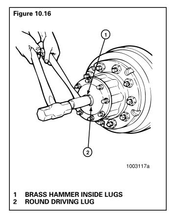
b. Hit the end of the drift with a large hammer (5 to 6 lbs, 2 to 3 kg) to loosen the axle shaft and tapered dowels from the hub. Figure 10.16. 8. Air Hammer Vibration Method:
