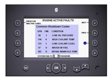
The list of common codes shown can cause engine shutdown and may be something that can be addressed onsite. Contact the engine manufacturer for information on other codes.
