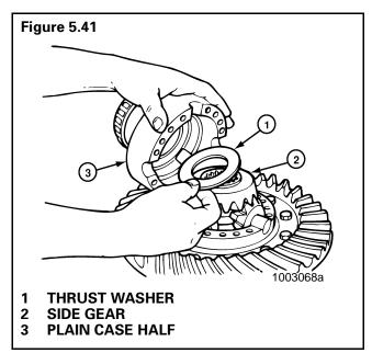
Place the plain half of the differential case over the flange half and gears. Rotate the plain half as needed to align the match marks.
