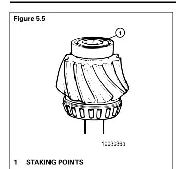
When using a staking tool and press (**Figure 5.5**), calculate the force required on the tool as follows.
