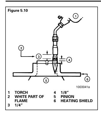
Remove the flame and the heat shield from the pinion. Let the pinion air cool for 10 minutes. Use a razor blade to remove the temperature indicating liquid.
