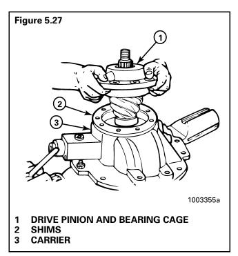
6. Install the bearing cage to carrier capscrews and washers. Tighten capscrews to correct torque value. Refer to **Table J. Figure 5.28**.
