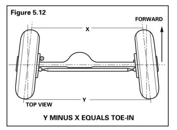
Check and adjust the toe setting after you install any of the following components:
