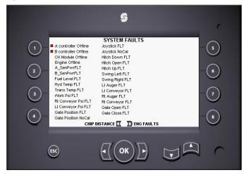
A red box will appear next to the problem that has been detected. An "Offline" fault means that there not CAN communication with the device. An input device fault (temp sensor, Pressure sensor, joystick or Gate position) indicates that the value at the input pin is above or below the specified range. This could be am open or short circuit to the
