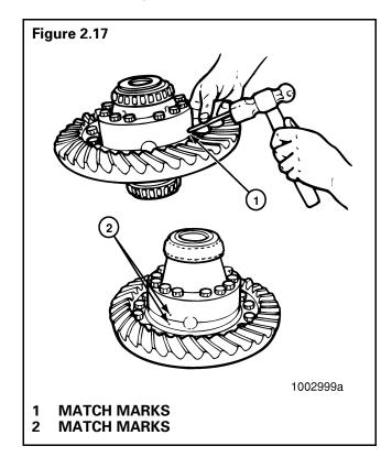
2. Remove the capscrews\* and washers\* or bolts\*, nuts\* and washers that hold the case halves together.
