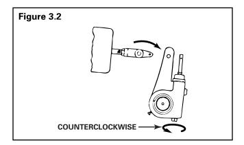
When you remove a clevis pin that has a spring, hold the spring with pliers. The spring can disengage from the clevis with enough force to cause serious personal injury.
