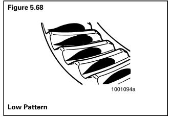
Look at the contact patterns on the ring gear teeth. Compare the patterns to Figure 5.66, Figure 5.67 and Figure 5.68.
