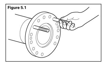
2. Apply a 0.125-inch (3.18 mm) diameter continuous bead of liquid gasket material around the flange mounting face of the axle housing.
