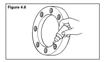
Tighten the fasteners to the specific torque value recommended for the fastener. Loctite<sup>®</sup> No. 277 will not alter the torque requirement.
