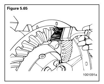
3. Rotate ring gear forward and backward so that the 12 gear teeth go past the drive pinion six times to get the contact patterns. Repeat if needed to get a more clear pattern.
