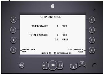
This screen displays the distance traveled while chip spreading Totals will only advance when the gate is open.
