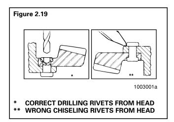
c. Press the rivets through holes in the ring gear and flange case half. Press from the drilled rivet head.
