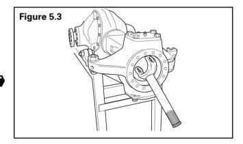
5. Install a new oil seal in the spindle bore. Apply a thin coat of NLGI grade 1 or 2 grease to the seal lips and bushing bore.
