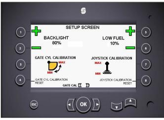
This screen is for setting brightness, low fuel level, Joystick and Gate cylinder input calibration.
