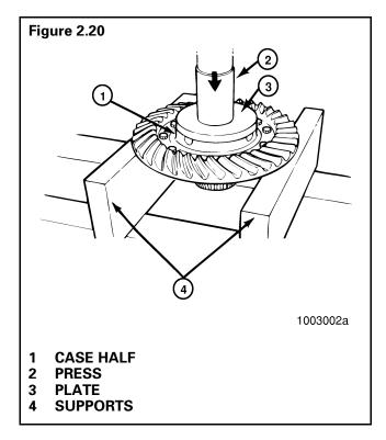
8. If the differential bearings need to be replaced, remove the bearing cones from the case halves. Use a bearing puller or press. **Figure 2.21**.
