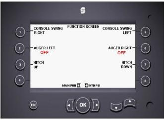
This screen has controls for the Console Swing, Augers (not available with CCH Hopper) and Hitch Up/Down.
