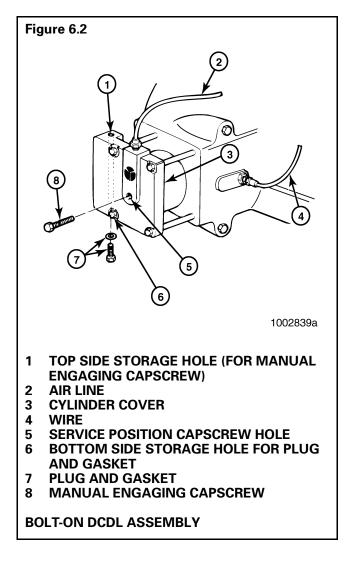
4. Install the plug and gasket into the bottom storage hole in the cylinder cover.
