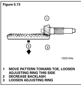
c. Repeat steps 2-4 and 6 until the contact patterns are at the correct location in the length of the gear teeth.
