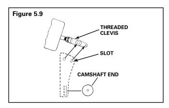
Verify that thread engagement between the clevis and push rod is 1/2-5/8-inch (12.7-15.9 mm). Figure 5.10.
