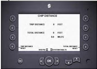
This screen displays the distance traveled while chip spreading Totals will only advance when the gate is open.
