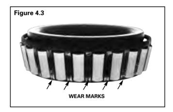
Damage on rollers and on surfaces of the cup and cone inner race that touch the rollers.
