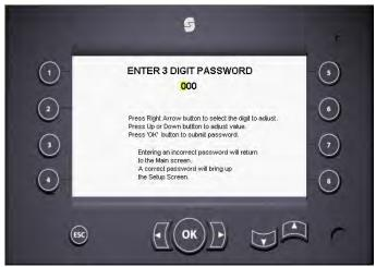
The Gate Calibration and Setup screens are password protected. The default password is **208**, but can be changed with the laptop service tool.
